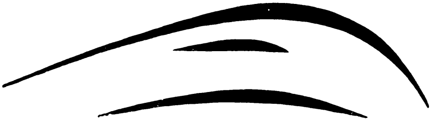
Fig. 96.—The arched wing sections discovered by Horatio F. Phillips and patented by him in 1884.
