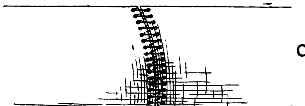
Fig. 129.—The mode of lacing the canvas on the upper plane.
