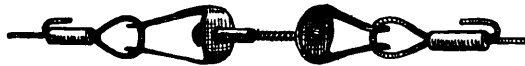
Fig. 158.—A simple rigging screw made out of a short cycle spoke and nipple, and two strips of metal.
