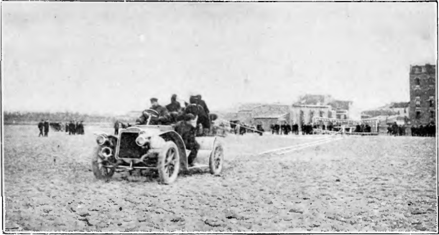
Fig. 57.—Experiments at Issy with a glider in 1900, power being obtained by towing the glider with a car.
