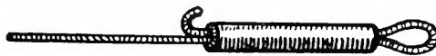
Fig. 112.—The general method of making eyes by passing the end of the wire twice through a piece of copper tube, leaving an eye, and bending the end of the wire over.
